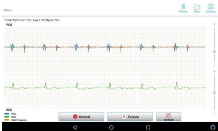
On tapping anywhere on the Record button, recording starts and the progress is indicated.
