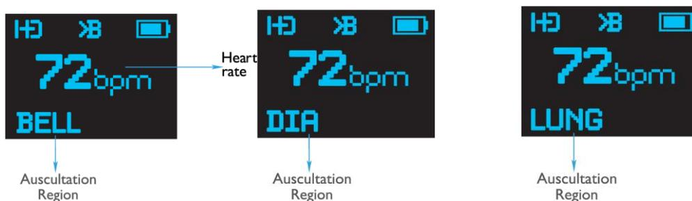
The BELL mode frequencies are from 50-200Hz. In this mode the user can hear low frequency sounds.
